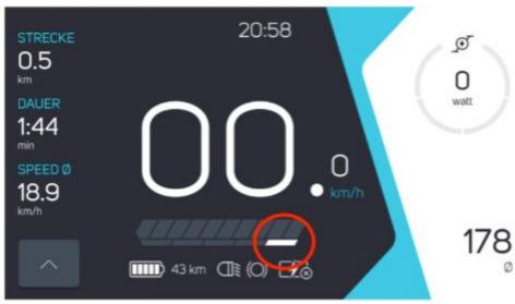
4. Reduce support level by two levels on tour, back on turbo and on tour again.
