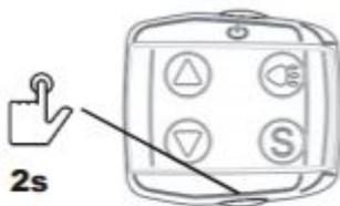
While driving (> 10km/ h), press the pushing assist button for 2 seconds.
