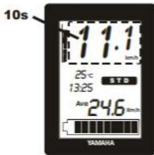
Speed 11.1 km/ h is displayed for 10 seconds.
