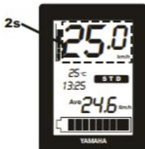
Display shows 25.0km/n for 2 seconds. Speed mode is off.
