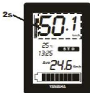
Dynamic mode on: 50. km/ h is displayed for 2 seconds.
