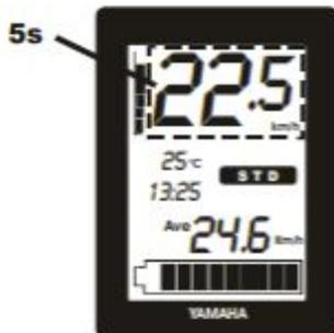
The wheel circumference stored in the drive unit is displayed for 5 seconds in centimeters. If necessary, adjust with the "arrow up" and "arrow down" buttons.
